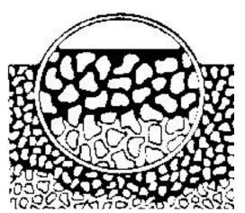
CONSEAL penetrates into the concrete where it reacts with free lime and alkali to fill the voids and bond the particles into a solid mass, creating a permanent seal.
