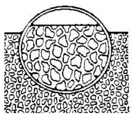
Spaces between particles leave untreated concrete subject to penetration by moisture, contaminates, oils, acids, etc.
