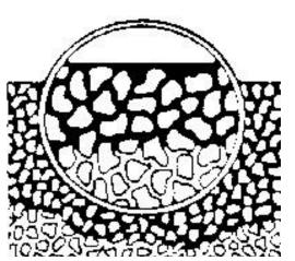
CONSEAL A-M 1000 penetrates into the concrete where it reacts with free lime and alkali to fill the voids and bond the particles into a solid mass, creating a permanent, integral seal.
